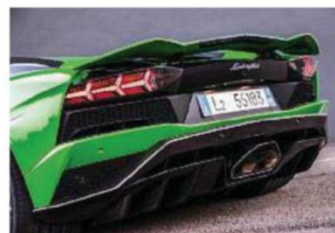
Aventador is now fitted with an active three position wing to aid downforce and stability
